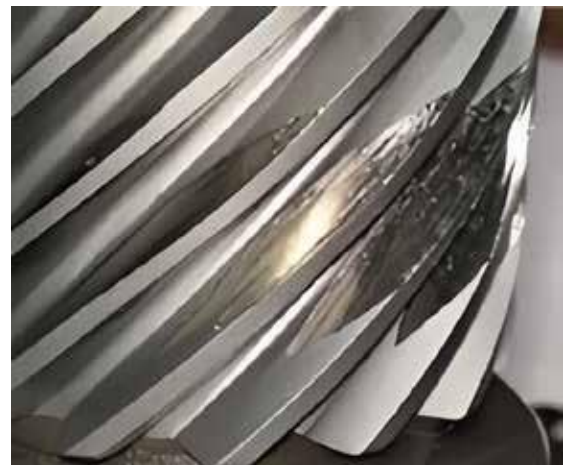
Figure 2: The tooth flank wear pattern of a crossed axis helical gear under excessive load (Courtesy of Indal Technologies, Curtiss-Wright division).
